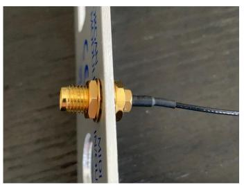
Insert the main board into the rear panel and tighten the nuts of the 6.3mm sockets.
