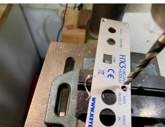
Center-punch the position and drill a hole with a diameter of 6.5mm.
