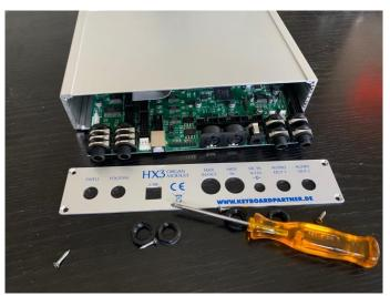
Pull the cover plate out of the grooves in the side panels.
