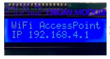
After switching on, the display now shows the IP address of the WiFi module 192.168.4.1.
