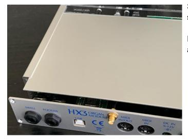
Screw the antenna onto the socket and point it upwards.
