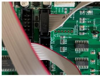
Solder the connector strip to PL33. The reverse polarity protection must point to the USB socket.
