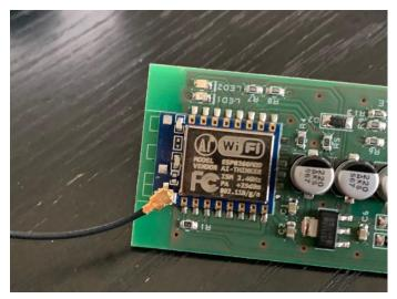
Remove the second protective film from the foam platelet, insert the WiFi module into the PL33 slot and press it onto the USB socket on the other side.
