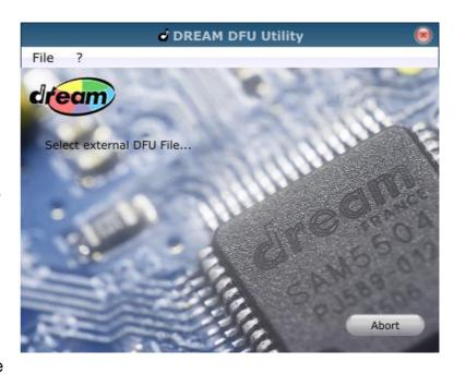
selection dialog opens where you can select the update package for your device. For a regular complete update select the file hx37 upd.dfu from the updates subdirectory. Wait until the unpacking is complete (displayed on the menu panel). Exit the DFU mode by restarting after the unpacking has been completed.
