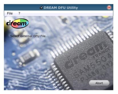
selection dialog opens where you can select the update package for your device. For a regular complete update select the file hx36\_upd.dfu from the updates subdirectory. Wait until the unpacking is complete (displayed on the menu panel). Exit the DFU mode by restarting after the unpacking has been completed.
