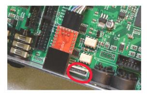
Remove four Philips screws on back and carefully pull out chassis a few inches. Insert two jumpers supplied with HX3 Drawbar Controller to jumper header PL10 of HX3 mk4 board or PL18 of HX3.5 board on positions 7-8 and 9-10 as shown in picture. Re-assemble back plate in reverse order and you're done.
