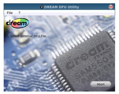
select the update package for your device. For a regular complete update select the file hx36\_upd.dfu from the updates subdirectory. Wait until the unpacking is complete (displayed on the menu panel). Wait until the unpacking is complete (displayed on the menu panel). Exit the DFU mode by restarting after the unpacking has been completed.
