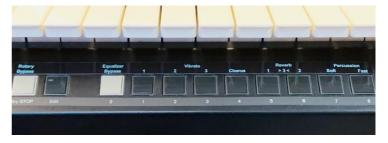
**Vibrato ON** switches vibrato on/off. Synchronously with the drawbar assignment, vibrato is switched to the lower manual when the LED in the Drawbars  $U \mid L \mid P$  button is lit.
