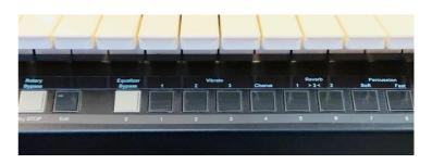
**Vibrato ON** switches vibrato on/off. Synchronously with the drawbar assignment, vibrato is switched to the lower manual when the LED in the Drawbars U | L | P button is lit.
