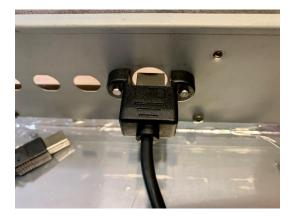
The USB socket is installed in the rear panel where the socket for the expression pedal was located. To do this, drill two 3 mm holes at a suitable distance (29 mm) close to the existing holes or enlarge them with a round file.
