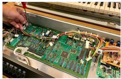
Disconnect all connectors and remove the large main board and the boards to the right of it.
