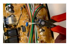
Remove all cable ties holding various harnesses together.
