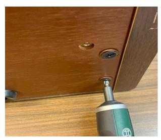
Loosen the 5 large screws on the bottom. Then the wooden lid can be removed.
