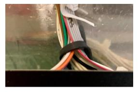
Fix the cables to the display and the buttons on the front tightly with the cable holder.
